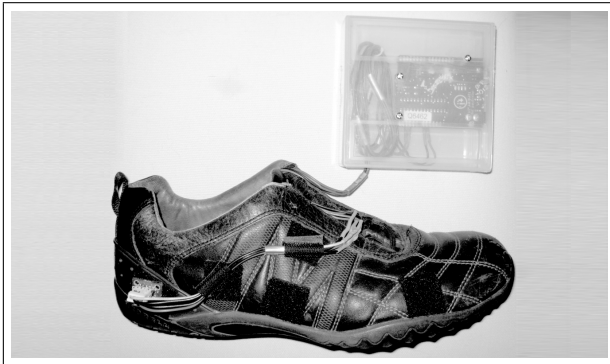
Figure 2. Prototype shoe/sensor system. The accelerometer is attached to the right-rear position of the shoe. Data passes from the sensor to the I/O board mounted in a project box.
